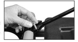
Position skyhook between arrows on label. When correctly positioned skyhook will be aligned to the center of the gen head and engine as shown.
